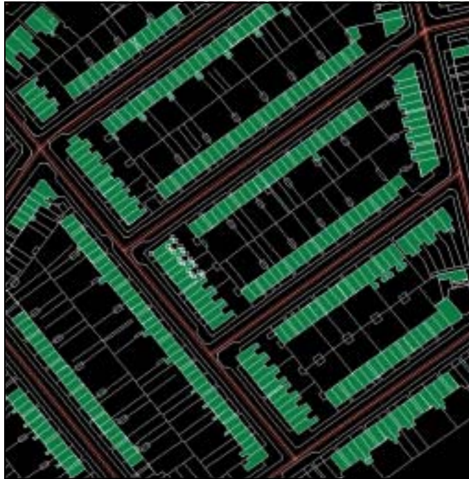
Fig. 6 An example showing the Lima concatenation function. The original AutoCAD® building information shown by white squares represents the back walls of the real buildings. Similar lines represent the front walls and the building separators. Lima converts them to separate buildings (coloured polygons with white border)
